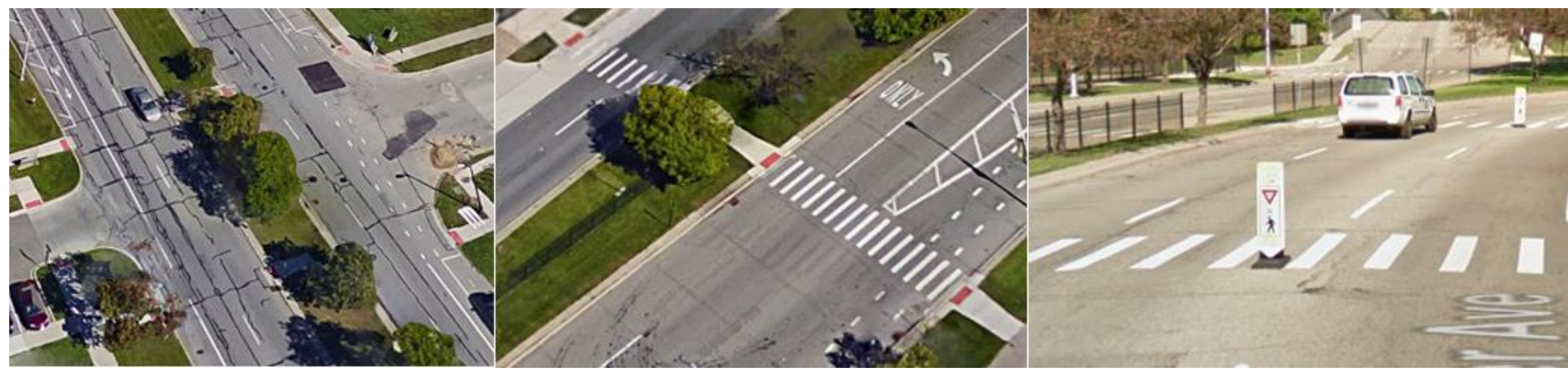
Figure 1. Three crosswalk types studied: from left, unmarked, continental markings, in-street R1-6 (images from Google Maps)
