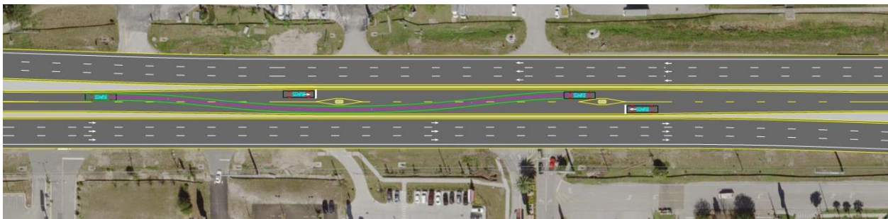
14 15 16 FIGURE 4 Bus overtake zone with contraflow operations
