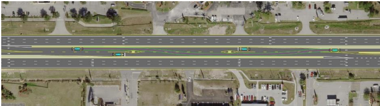
18 19 20 FIGURE 5 Bus overtake zone with conventional flow operations
