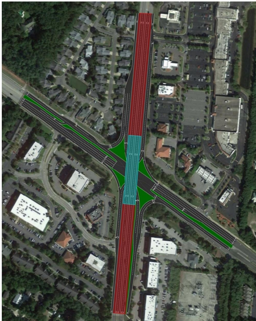
FIGURE 2 – Geometric Layout of SPUI along Military Cutoff Road.
