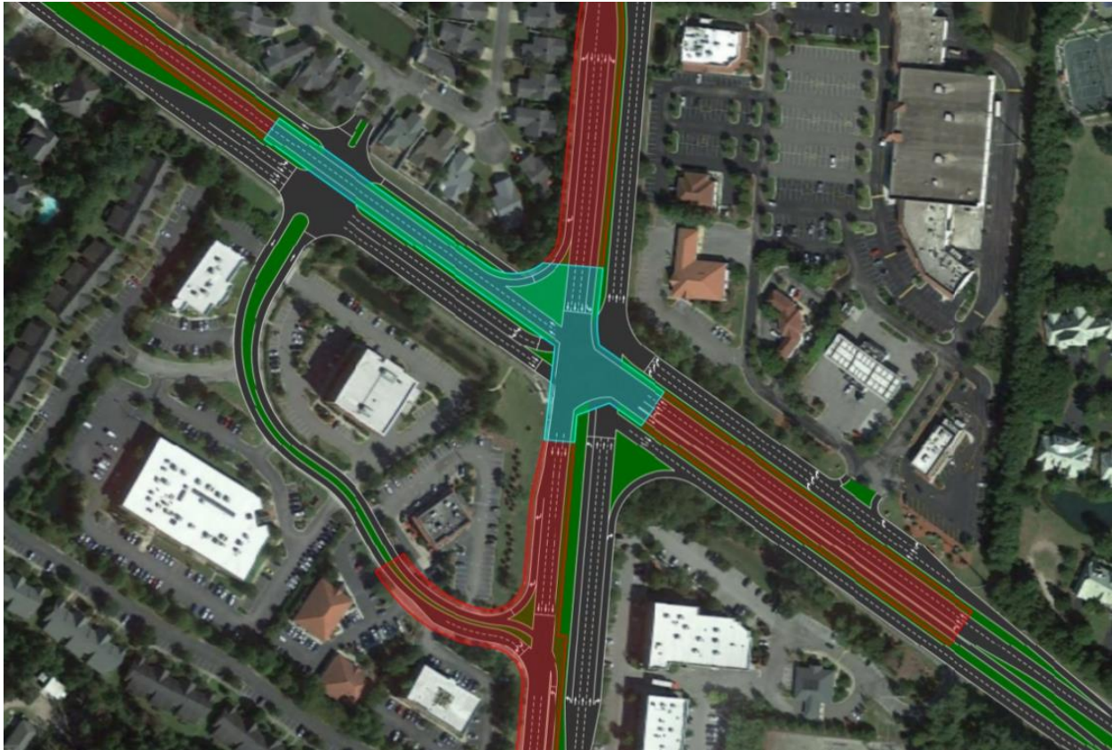
FIGURE 5 - Geometric Layout of Echelon.
