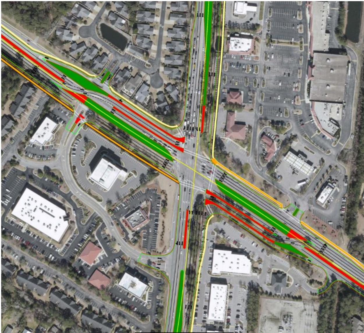
FIGURE 9: Geometric Layout of CFI along Eastwood Road.
