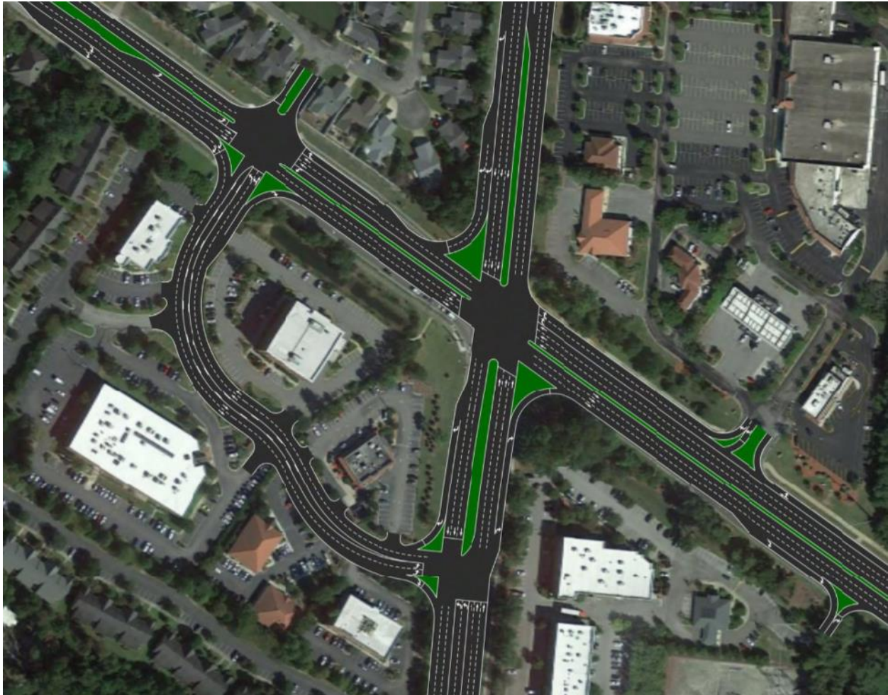
FIGURE 6 - Geometric Layout of Quadrant Road at Grade.
