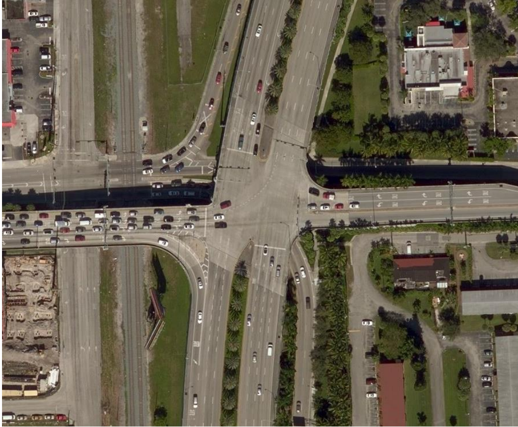
FIGURE 4 - Example of an Echelon Intersection in Aventura, FL.
