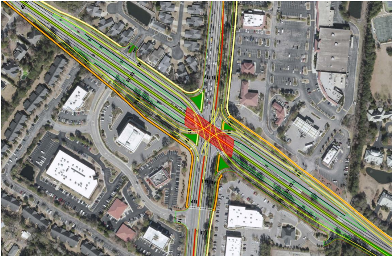
FIGURE 3 – Geometric Layout of SPUI along Eastwood Road.
