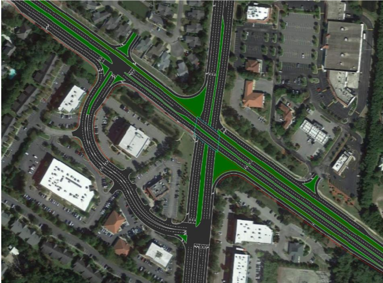
FIGURE 7 - Geometric Layout of Quadrant Road with Overpass.
