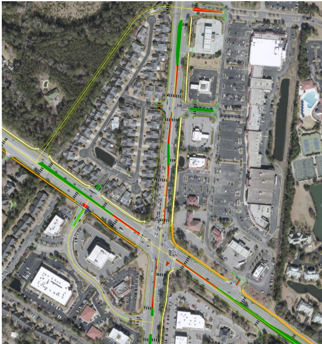
FIGURE 10: Geometric Layout of NW Quadrant Road.
