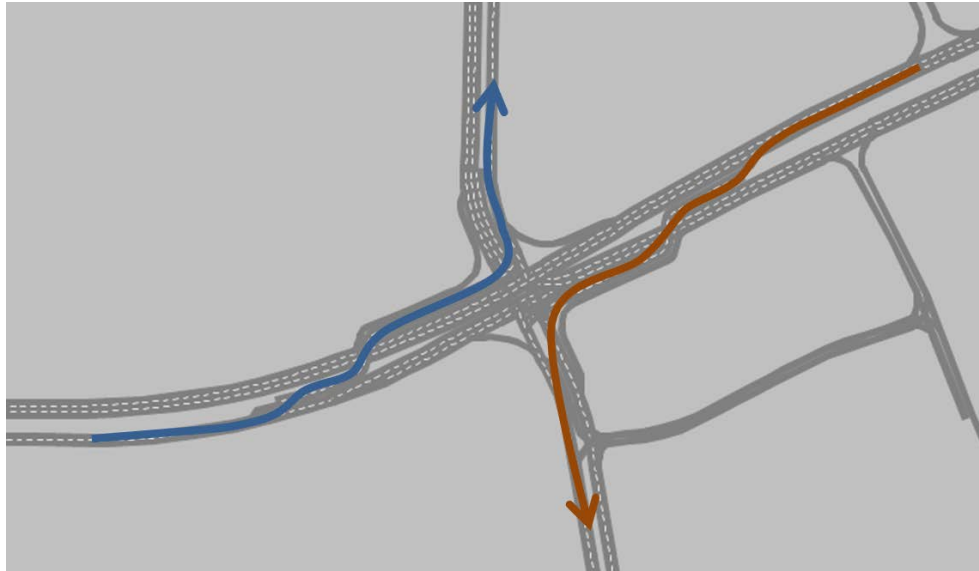
Figure 4 Partial continuous flow intersection layout at N Commerce Dr.
