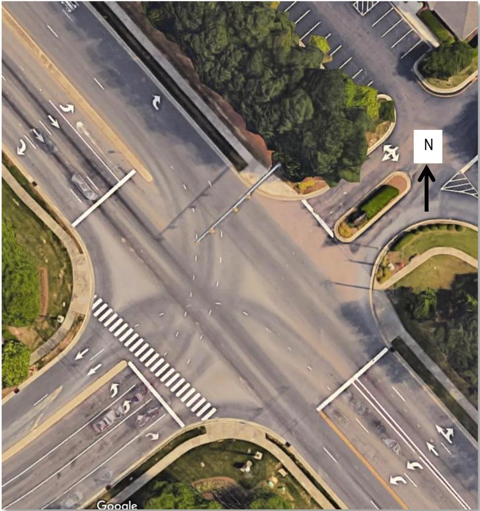
Figure 4. Lane discontinuity in Apex, NC resulting in poor lane utilization (Google).
