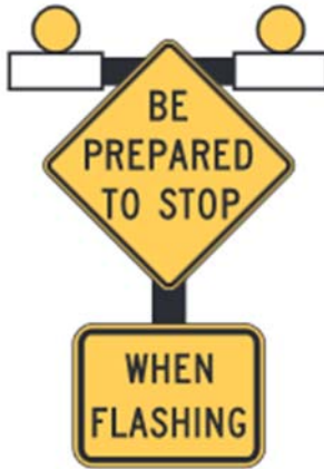
1 2 FIGURE 14 Be Prepared to Stop (W3-4) sign and When Flashing (W16-13) plaque with 3 beacons. (9) 4
