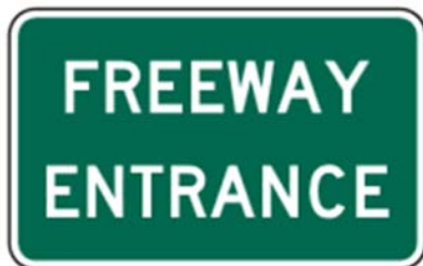
25 26 FIGURE 12 Freeway Entrance (D13-3) sign. (9) 27
